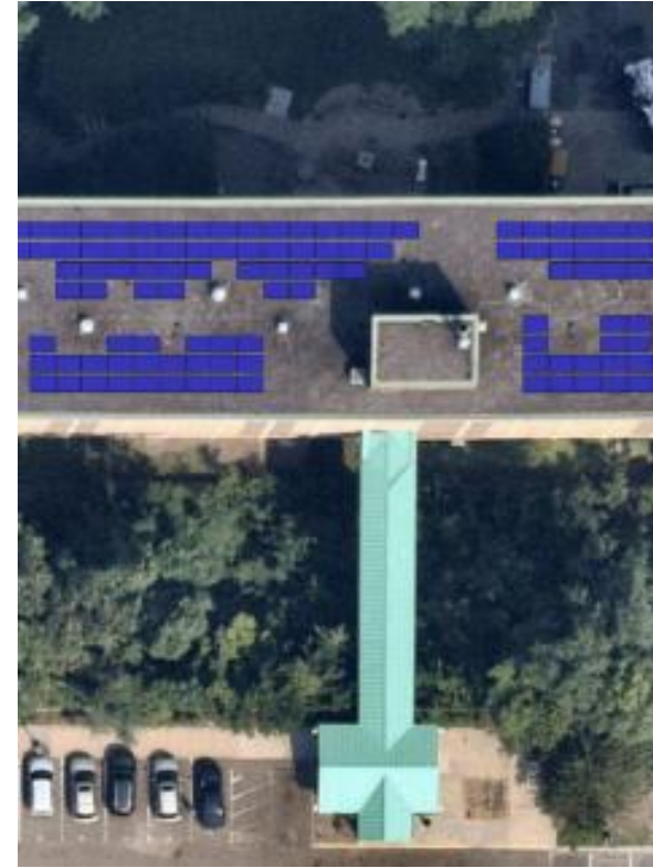
Projected solar installation on Nan McKay to help offset electrical load with renewable energy.
